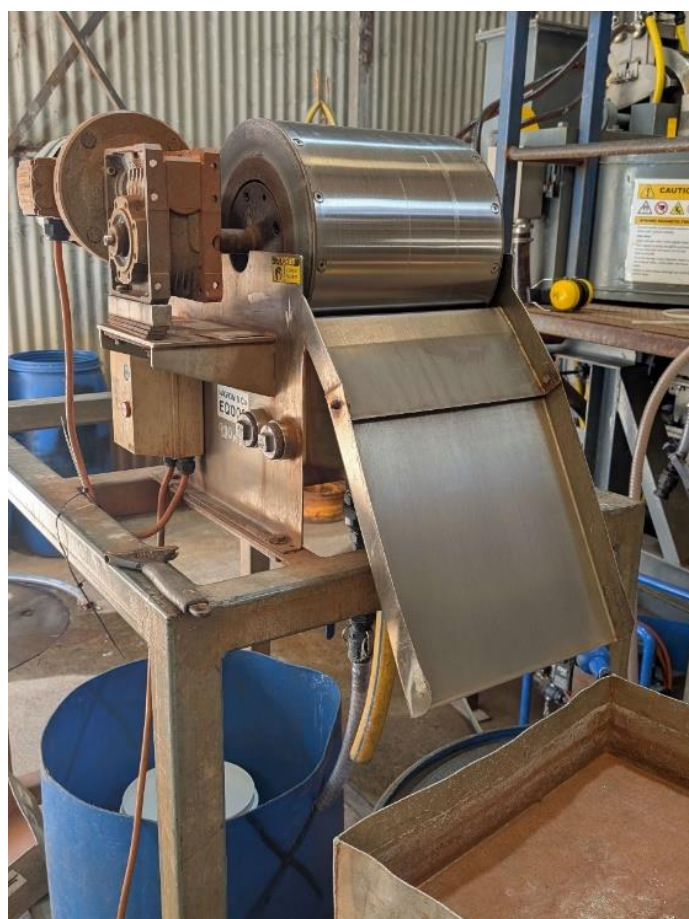
Plate 1: Low Intensity Magnetic Separation (LIMS); NAGROM Laboratories.
