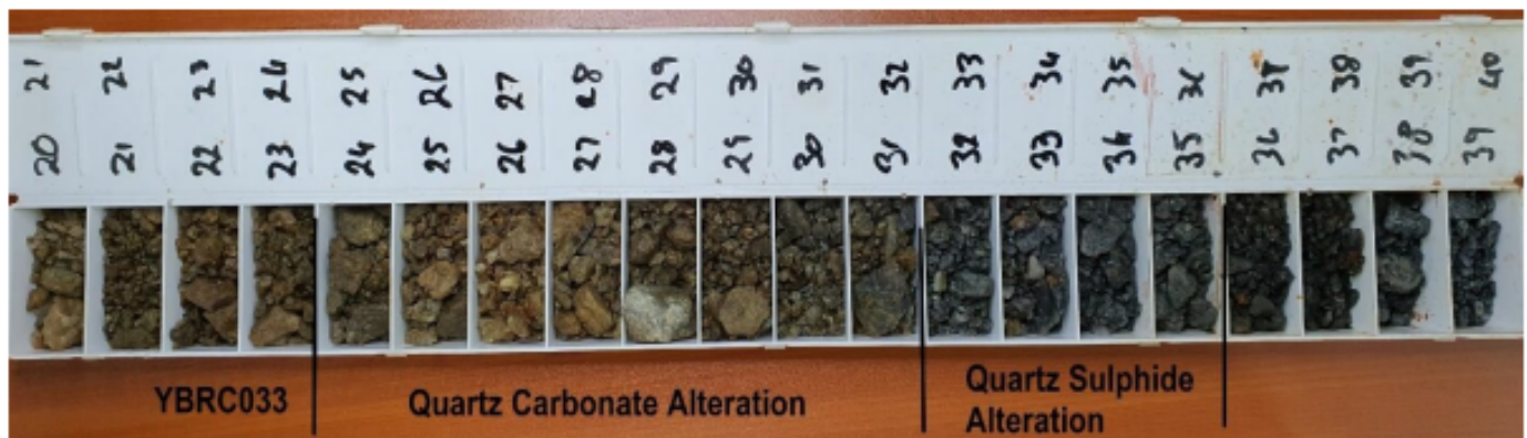
RC drill hole YBRC033 showing 12m quartz-carbonate-sulphide alteration
